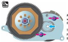
Adjust the motor so the pinion meshes with the spur gear properly. Make sure the gear mesh is not too tight.
