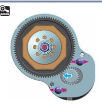
Adjust the motor so the pinion meshes with the spur gear properly. Make sure the gear mesh is not too tight.
