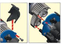
To remove the motor, first open the right battery door and slide out the ESC. Next, remove the single large hex screw using the supplied 2.5mm wrench. Then rotate the motor and mount to the side of the model, and slide backward off the post.
