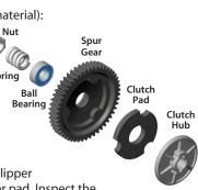
tightened, disassemble the slipper clutch and replace the slipper pad. Inspect the spur gear and pressure plate for wear or damage and replace if necessary.
