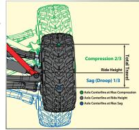
ground clearance is needed. However, the vehicle's center of gravity (CG) will be raised, making it less stable.
