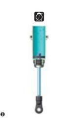
Orient the filled shock vertically for several minutes with the shock shaft fully extended. The remaining air bubbles will release.
