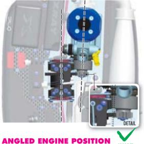
CORRECT Please note that the engine is not parallel with the chassis centerline, so that the clutchbell engages the spur gear at a slight angle. This is correct and will not have any effect on handling, performance, or lifespan of any parts.
