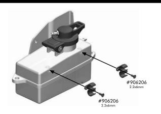
Tube holders are easy connected to the fuel tank by screws. The main advantage of this system is that the holders will never fall down as could happen when the glue is used.
